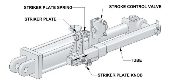
If you intend to use full extension of the cylinder, simply unscrew the striker plate knob and move the striker plate away from the valve to the very end of the adjustment tube, then retighten the knob.
